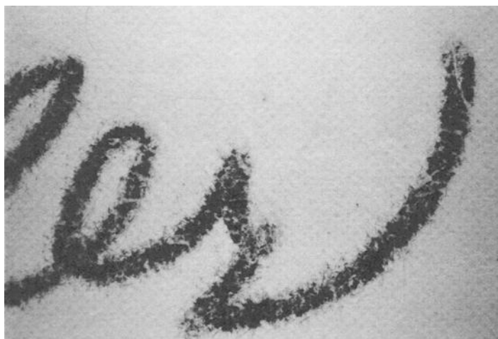
FIG. 12 a — Carbon traced signature ( \times 10 magnification). The carbon particles are forcibly embedded in the fibers of the paper.
