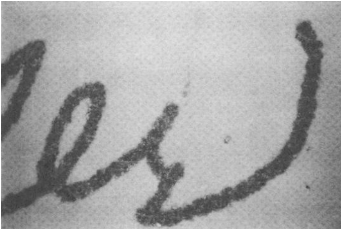
FIG. 11a— Gelatin transfer signature ( \times 10 magnification). The fibers of the paper appear to be thoroughly dyed. The color is diffuse and not as crisp as the genuine stamped facsimile signature. The trash carbon particles carried over in the transfer process have a tendency to bleed into the paper or slightly dissolve and lay upon the paper surface.
